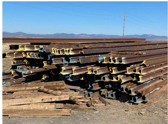
Picture of one batch of 119-lbs rail in yard. Blue ends are 39'-40' rails, yellow are 36'-39'
